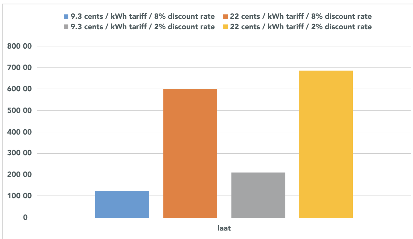
Figure 11. Annual savings from the installation of solar PV in laot WWTP (USD)
